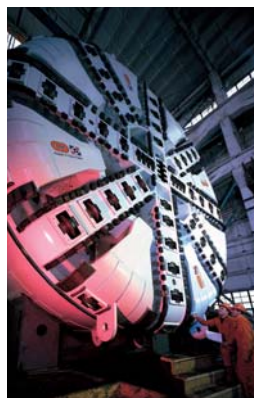
Mixed ground earth pressure balanced Tunnel Boring Machine
